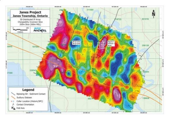
Figure 3: 3D Distributed IP Array Chargeability Inversion Slice (200 m) of the Janes Property with interpretations and drill hole locations. Historic drill collars are represented with red diamonds while the 2021 drill collars are represented by the blue diamonds. Note: For the survey, an average sea level (Mean Sea Level - MSL) of 300 m was used.
