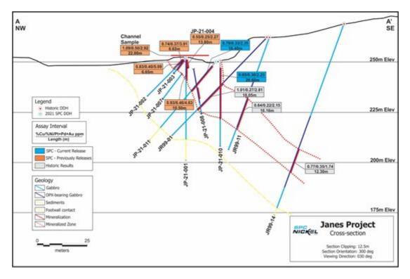
Figure 2: Cross section of the Trench 1 area along A-A' (refer to Figure 1). Section is orientated at 300°
